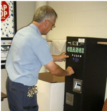
The locks are programmed with route information via a special key. There can be an unlimited number of locks on any route. If a machine is changed to a different route you need only touch the change key to the lock to update its route information. The lock does not need to be removed from the vending machine.
